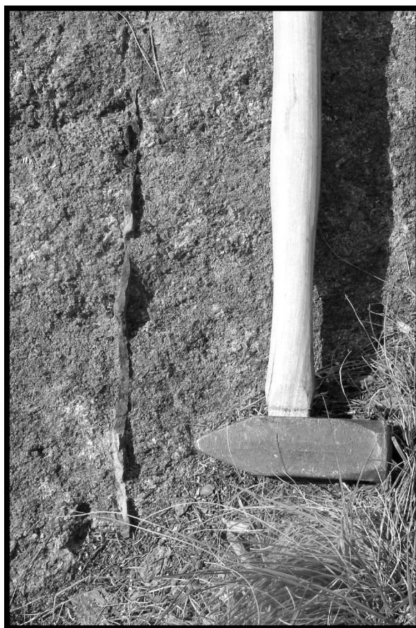
FIGURE 3 —Vertical rusty quartz vein in felsic gneiss located ~10 meters south of Bald Mountain fire tower. Vein is approximately 8 mm wide. Hammer for scale.
