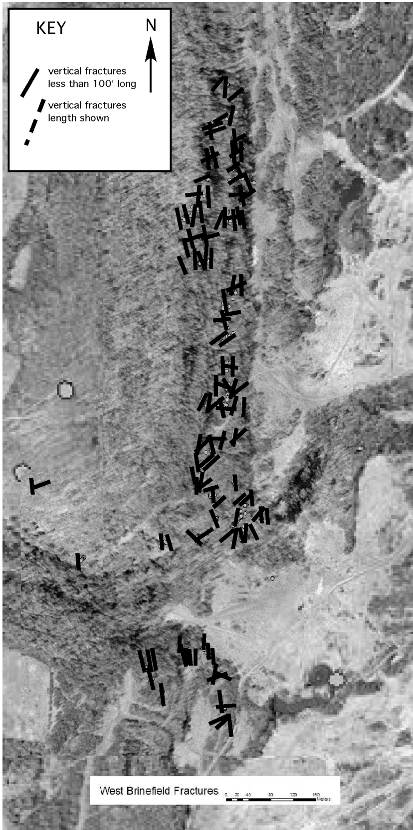
FIGURE 4—Aerial photo of the West wall of Tully Valley showing distribution of fractures.
